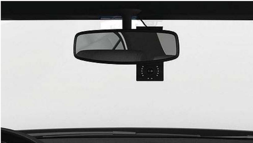
The idrive mounting base will adjust to accommodate any angle windshield.
